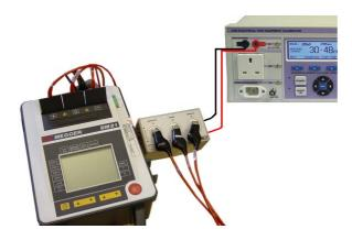
Note the maximum voltage rating of 1kV on the 3200 does not allow 5kV testers to be directly calibrated with the 3200.
